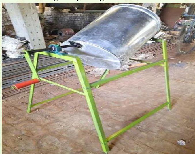
Figure 3: Seed Treatment Drum for uniform chemical mixing in seed preparation.
